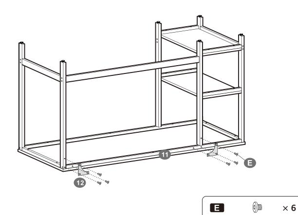
After assembly, please check all screws and adjust the leg leveler to ensure stability.
