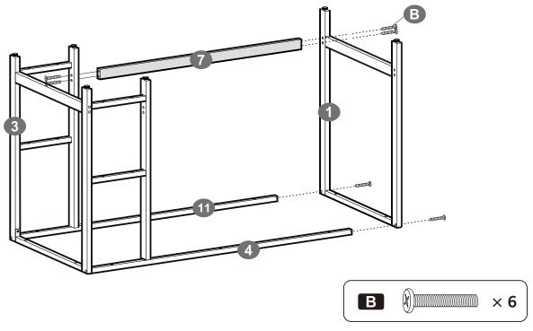
Do not tighten the screws all at once so that board can be adjusted slightly. Align all screws to the corresponding pre-drilled holes first and then tighten them one by one.
