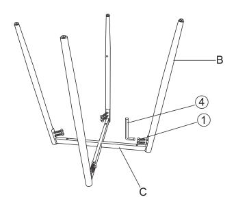
Attach the Leg (B) to the Cross Connection (C) using the Bolts (1) with Allen Wrench (4) as pictured above.
