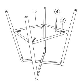
Attach the Square Connection (D) to Leg(B) using Bolts (2) with Allen Wrench (4) as pictured above. Do not fully tighten the Bolts.
