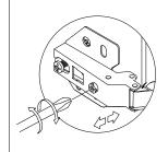
This is used to adjust the door panel in the left and right direction.
