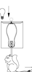
Step 2 Insert the bulb(G) into the socket(C).
