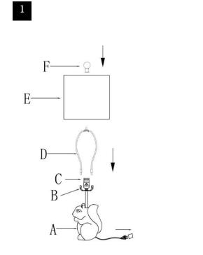
Step 1 Insert the Harp (D) into the Saddle (B). Put the shade(E) on the Harp(D), then tighten the Finial (F)into the Harp (D)
