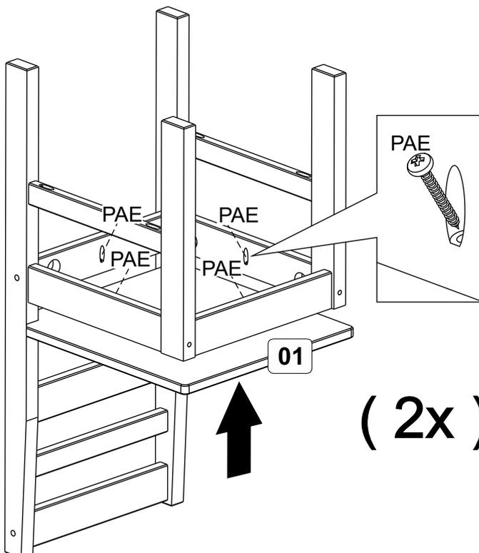
\* Place the seat base (part 1) on a clean work top or other flat surface, use a soft cover to protect the surfaces and position the built chair frame upside onto the base, check the frame is positioned centrally before fastening to the base.
