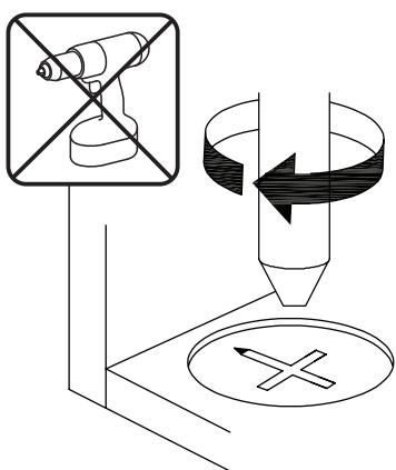
**EN**\_Turn cam lock clockwise to tighten.
