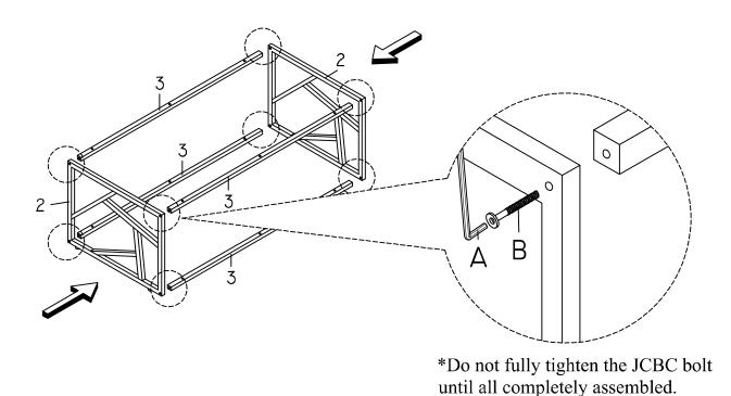
Attach top panel (1) & fixed panel (4) to metal rail (3), JCBC screw (B), tighten by using allen-key (A).
