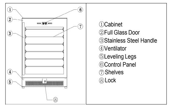
Note: EL-WCU103-02 or EL-WCU105-02 is with right hinge, the handle is on the left. EL-WCU110-02 or EL-WCU1112-02 is with left hinge, the handle is on the right.
