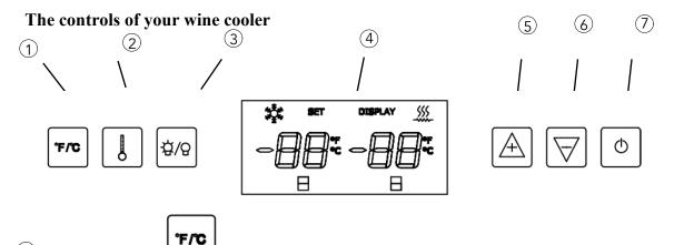
① °F/°C Selector Select the temperature display setting in Fahrenheit or Celsius degree.
