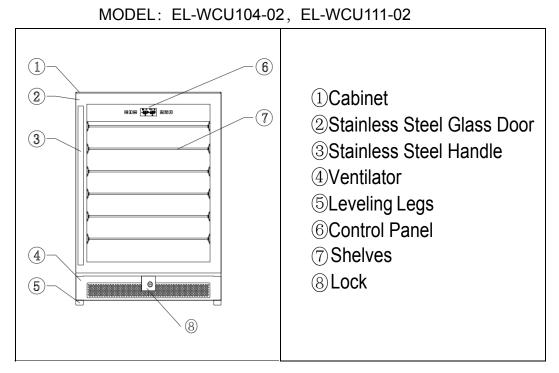
Note: EL-WCU104-02 is with right hinge, the handle is on the left. EL-WCU111-02 is with left hinge, the handle is on the right.
