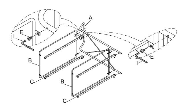
2 Attach Shelf Ring (B) & Cross Bar (C) to the other piece of Side Frame (A) using Bolt (E) by Allen Key (I) as below shown.
