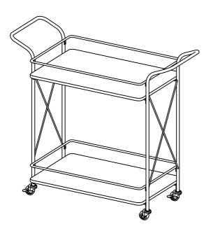
This page lists all the contents included in the box. Please take the time to identify the hardware as well as the individual components to this product. As you unpack and prepare for assembly, place the contents on a carpeted or padded area to protect them from damage. 1 Attach Shelf Ring (B) & Cross Bar (C) to one piece of Side Frame (A) using Bolt (E) by Allen Key (I) as below shown.
