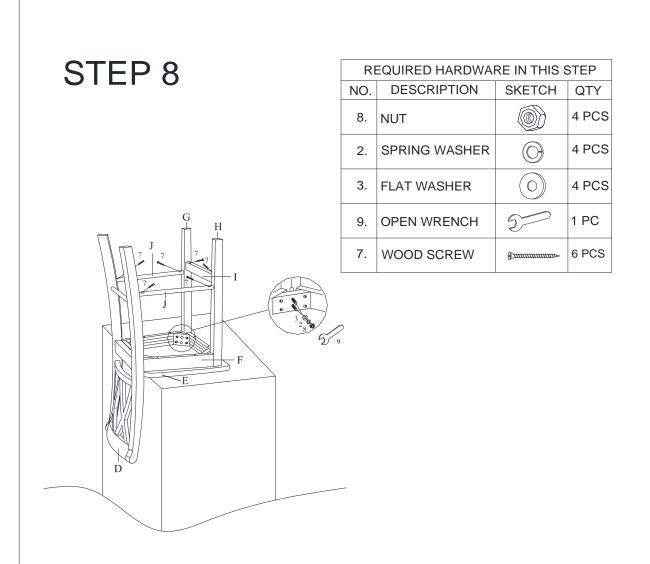
Attach chair left and right front legs (G & H) to seat frame (F) with flat washers (3), spring washers (2), and nuts (8) as shown. Do not fully tighten nuts (8). Insert chair left side crossbar and chair right side crossbar (J) into the front left and right chair legs (G & H) and chair back frame (D).
