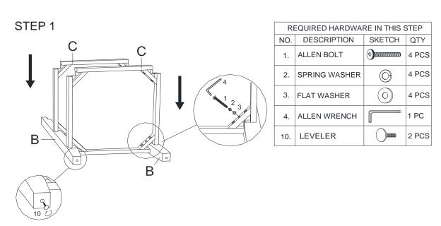
Attach table shelf (C) to the table legs (B) using Allen bolts (1), spring washers (2) and flat washers (3) as shown. **Don't tighten all Allen bolts at this step**.
