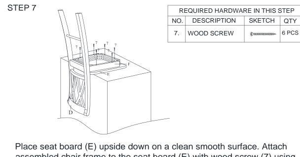
Place seat board (E) upside down on a clean smooth surface. Attach assembled chair frame to the seat board (E) with wood screw (7) using a Phillips head screw driver (not included).
