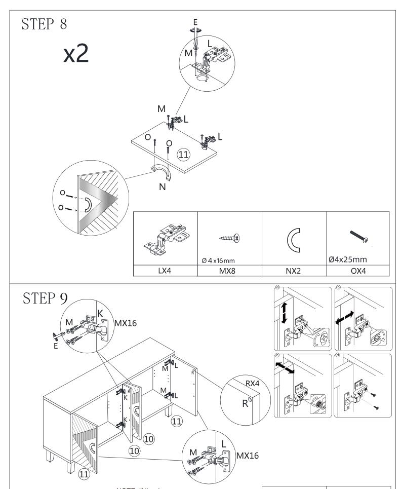
NOTE: If the doors are uneven or there is a gap in the middle, loosen or tighten the screw on the door hinge until they are sitting flush.
