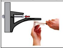
You will line up the bracket with the pre-drilled hole on your frame and insert the screw through the front into the nut on the back like shown here. A good snug fit is satisfactory, you don't want the bracket to be able to move once tightened.
