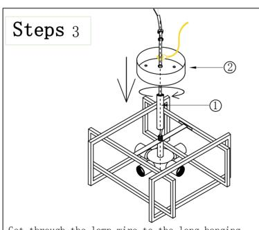
Get through the lamp wire to the long hanging rod, and screw hanging rod to the light fixture. Get through the lamp wire to the canopy, and installation ground wire is fixed by screws.
