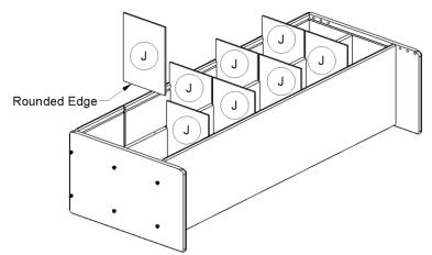
5. Insert 2-Backs-**I** by inserting into LH Side groove on one end, bowing into other groove on opposite end, and sliding into full length grooves on Top and Bottom.
