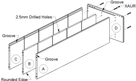
3. Install <u>RH-Side</u>-**E** by aligning dowels. Ensure back groove is up and aligns with other grooves. Loosely install with 6-XAUR Decorative Screws with 4mm Hex Wrench provided.
