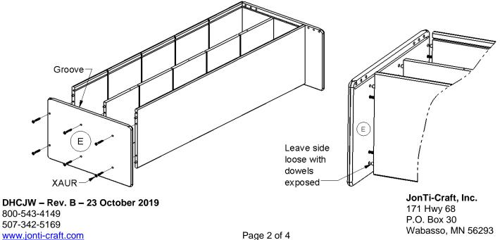
4. Drop in 8-<u>Hardboard Dividers</u>-**J** into groves with rounded edge down.
