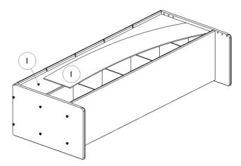
6. Install <u>Hanging Bracket</u>-**F** and <u>Hook Rail</u>-**G** by aligning dowels. Ensure Backs (previously installed) are seated into Top, Bottom, and Side grooves. Note location and orientation of mitred edge of Hanging Bracket and hooks on Hook Rail. Tighten 6-**XAUR** Decorative Screws previously installed.
