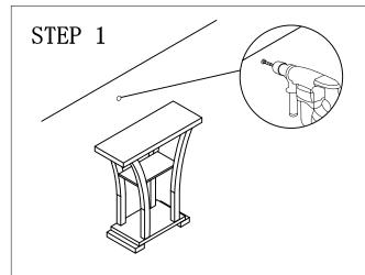
To drill a hole (about 1") on the wall.
