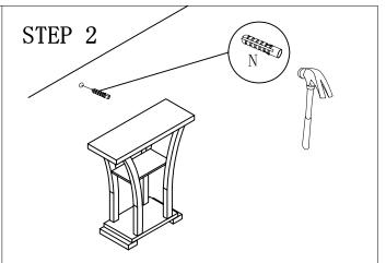
To tap drywall anchor into the hole.
