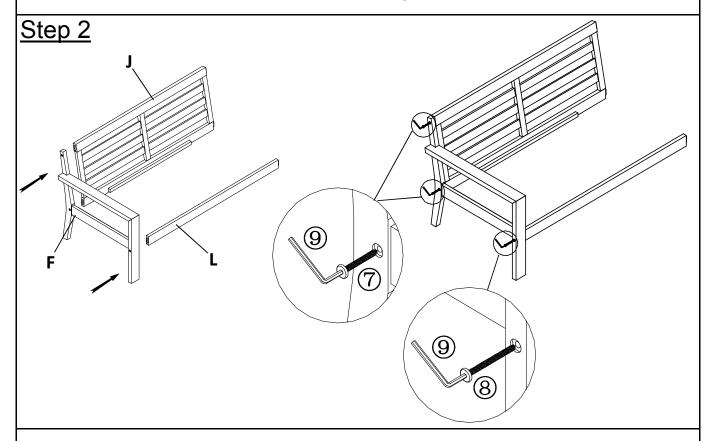
With the help of your adult partners, attached the tenons of Backrest Panel (J) and Support Bar (L) into the mortises of Left Panel (F) using Bolt (7) and (8) with Allen Key(9) as shown in picture above.
