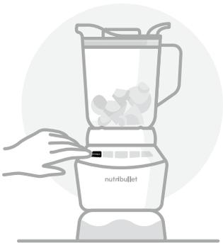
To start blending, select a speed or the **EXTRACT** program on the blending control panel. This program will turn off automatically. Buttons will illuminate while in use.
