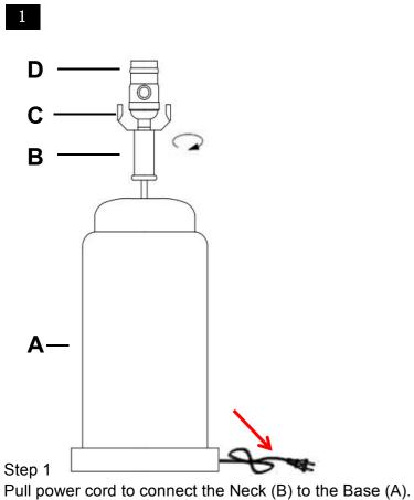
Pull power cord to connect the Neck (B) to the Base (A). Screw the Neck (B) onto the Lamp base (A) Be careful not to twist the power cord and tighten securely
