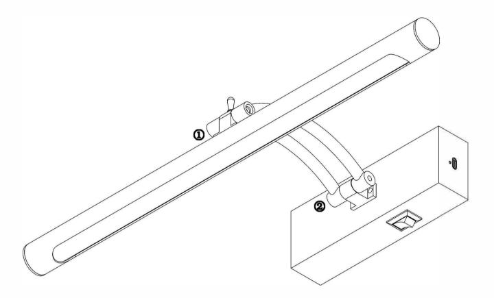
**ATTENTION:** During the transportation, the screws at the connection ① and the universal head ②may be a little loosened, you can use household screwdriver and tighten the screws to retain itsposition, according to your needs.
