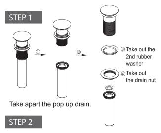
Insert the drain top into the vessel. Install the thick rubber washer and then the drain nut. Tighten the drain nut and then the tall piece.
