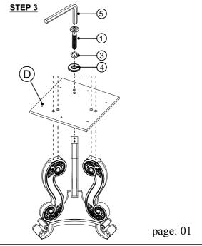
\*\*\* Do not fully tighten screws until fully assembled \*\*\*
