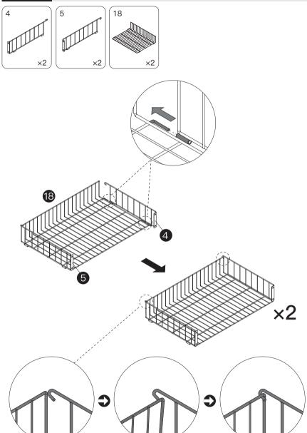
Note: Bend the frame to connect each other when necessary.
