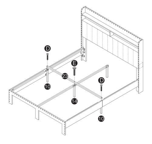
Step 17 Install part (6) and part (7) on the frame, align and fix the Verclo, use part (5) to tighten part (6).
