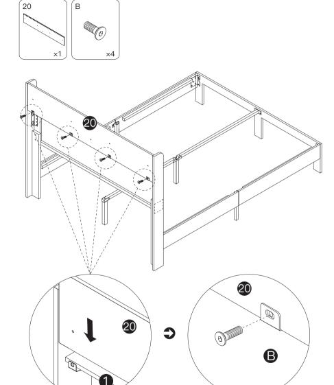
NOTE: Tighten all the screws (part f B) after installing part  $f 2\!\! 0$ .
