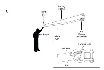
WARNING: RAISING THE FRONT BAR WILL REDUCE THE PITCH (ANGLE) OF THE FABRIC THUS INCREASING THE RISK OF RAIN WATER POOLING ON THE FABRIC. TO PREVENT THE AWNING FROM COLLAPSING DUE TO RAIN WATER LOAD, YOU MUST RETRACT THE AWNING WHEN UNATTENDED. FAILURE TO DO SO COULD RESULT IN PERSONAL INJURY.
