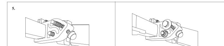
Step5. Then insert the big arm side into arm shoulder bracket and fasten the two locking nuts.
