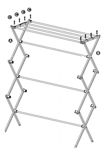
5. Insert the top 4 bars (C) one-by-one, inserting both ends of each bar at the same time.
