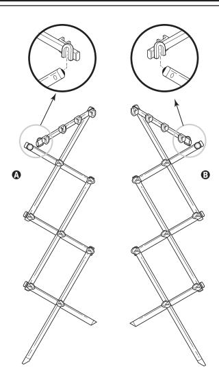
1. Open each frame side support fully, press each top horizontal bar end into connector to secure as shown.
