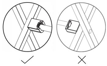
\* Please make sure all ends have been inserted into U-shaped channels by gently pushing each one.
