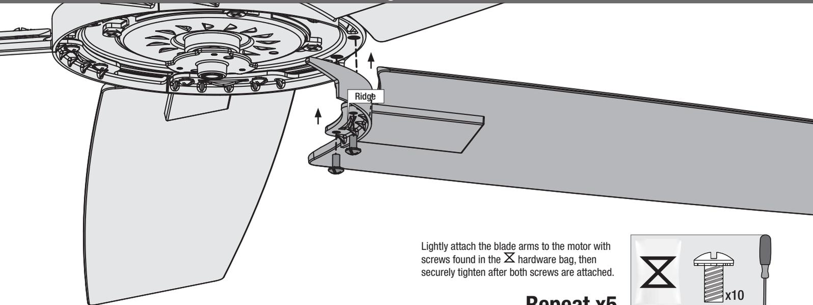
Lightly attach the blade arms to the motor with screws found in the ✕ hardware bag, then securely tighten after both screws are attached.
