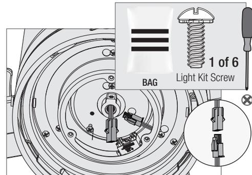
Insert the third screw, found in the hardware bag, into place and then tighten all three screws. Connect 3-pin to the plug connector found in the switch housing area of the light kit assembly. Make sure to line up the colored markings on the connectors.
