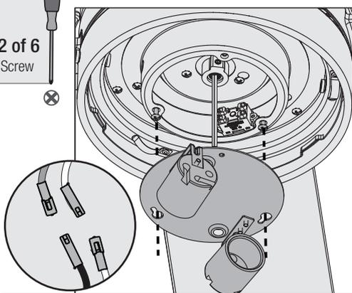
Lift the light kit and connect the single-pin connectors to the connectors from the fan. Connect the white wires together. Connect the blue and black wires together. Align the keyhole slots in the light kit housing with the two screws. Make sure all the wires from the fan and the light kit are snug inside the center of the light kit, not pinched in between the upper switch housing and the light kit or hanging out of the sides.
