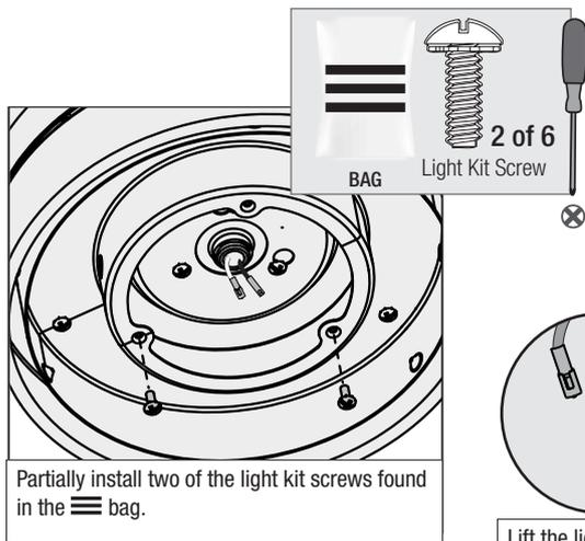
Partially install two of the light kit screws found in the bag.
