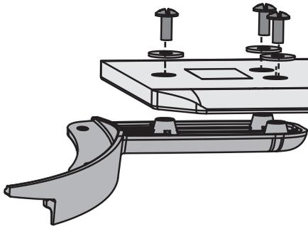
Put the blade washers, found in the ■ hardware bag, onto the blade screws, found in the ▲ hardware bag. Then install the blade screws to secure each blade to a blade iron.
