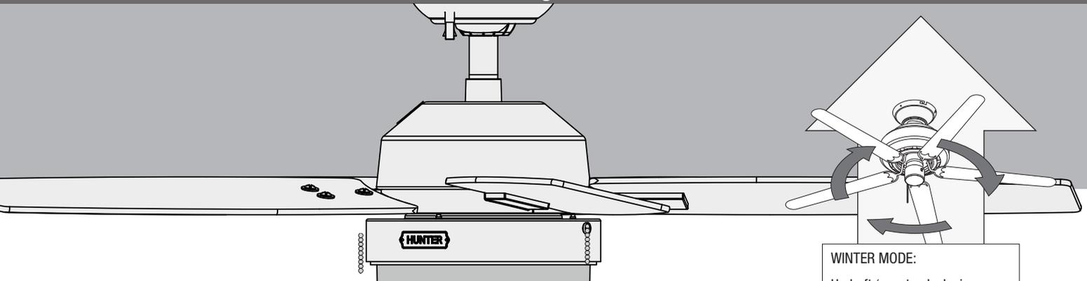
Ceiling fans work in two directions: downdraft (counterclockwise rotation) and updraft (clockwise rotation). To change the fan's rotation direction, wait until the fan comes to a complete stop (audible triple beep). Then pull the fan chain and continue to hold it until you hear a double beep. This double beep indicates that the direction has been successfully changed.
