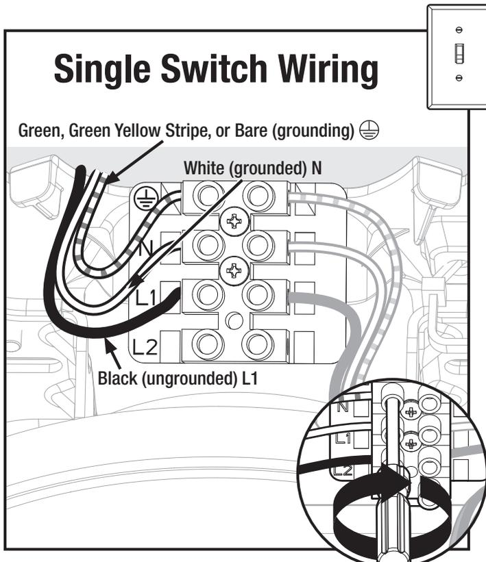
Connect wiring from ceiling to terminal block (on side of canopy mount) and tighten using flathead screwdriver (included).
