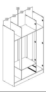
**Step 9:** Attach the top panel (1) using hardware parts C and D with a screwdriver (not provided). Secure the back panels (23) using hardware parts I, Q, V and U with a small mallet and screwdriver (not provided).
