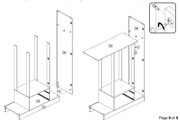
**Step 7:** Secure the shelf (2) to the supports using hardware parts C, D and P. Position the hanging rain (24). Attach the left panel (4) using hardware parts C and D. You will need to use a screwdriver (not provided). **DO NOT use any power tools as this may damage the frame and will invalidate any claim.**
