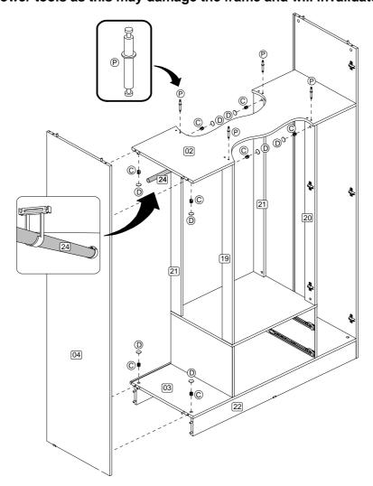
**Step 8:** Attach the shelf dividers using hardware parts C and D with a screwdriver (not provided). Connect two back panels (23) together with the spine (25) and position.
