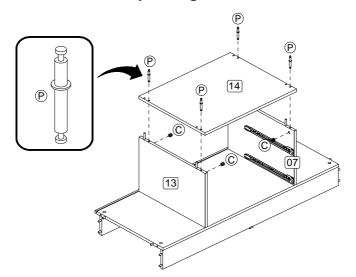
**Step 5:** Attach the supports using hardware parts C and D with a screwdriver (not provided). **DO NOT use any power tools as this may damage the frame and will invalidate any claim.**
