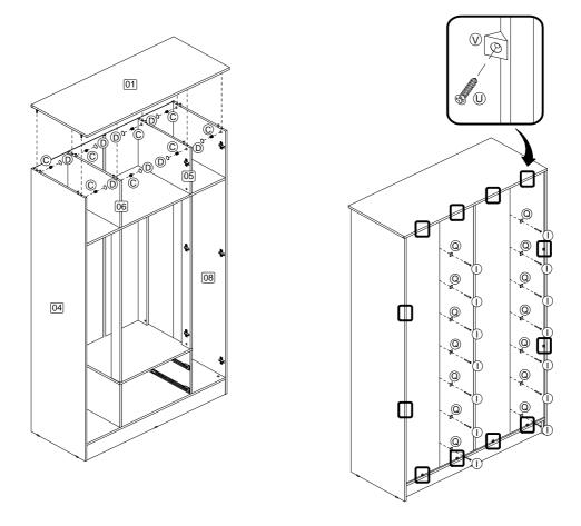
**Step 10:** Attach the doors as shown, then attack the handles (26) using harware part F. Youwill need to use a screwdriver (not provided).
