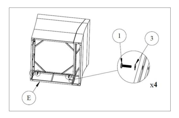
5.Align Plastic Leg (5) to the frame body by the pre-drilled threads with Bolts (1). It should have 4 plastic legs and 8 bolts fastened. Tighten all bolts. (Photo 5)
