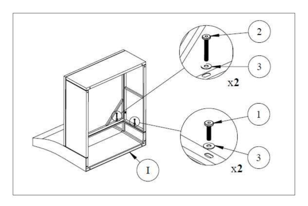
3.Align Plastic Leg (5) to the frame body by the pre-drilled threads with Bolts (1). It should have 4 plastic legs and 8 bolts fastened. (Photo 3)
