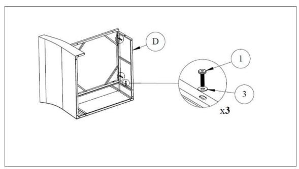
4.Position Front Frame (E) and frame (3) by the pre-drilled threads. Use Allen Key (4) to fasten Bolts (1) with Washers (3). It should have 4 bolts fastened. Do not tighten bolts. (Photo 4)
