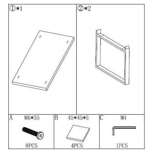
Step 1: Lay the Table Top(1) upside down onto a clean smooth surface such as carpet or cardboard. Align and fix two table legs (2) to the Table Top(1) with 8 pcs screw(A) by Allen Key(C).Do not fully tighten all bolts until all parts are in place.
