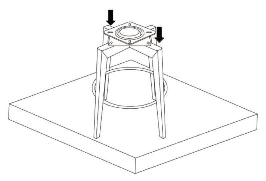
6 Attach the assembled stool base in Step 5 to the Seat Bucket (C), using Short Bolts (H2), Lock Washers (H3), Flat Washers (H4) and Allen Wrench (T1). Fully tighten all bolts.
