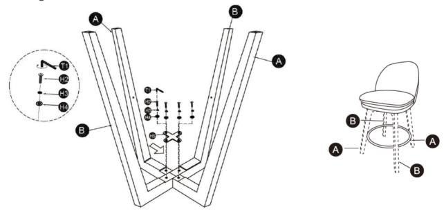
Flip over the stool base. Loosely attach the Long Bolts (H1) one by one and keep them loose. Do not fully tighten. After loosely attach the first bolt, move on to the diagonal bolt. After all 4 bolts are attached, use Allen Wrench (T1) to tighten.
