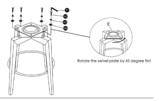
**5** Put assembled stool base in Step 4 on a flat surface. Push legs up or down as necessary to level. Once level, fully tighten all bolts.
