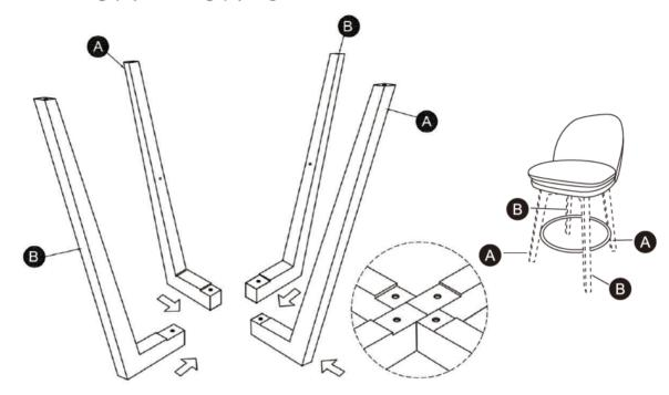
Place the cross metal plate (H5) in the middle of the stool base. Proceed to loosely attach the Short Bolts (H2) one by one, but keep them loose. Do not fully tighten them yet. After loosely attaching the first bolt, continue with the remaining bolts. Once all 4 bolts are attached, use the Allen Wrench (T1) to tighten them.
