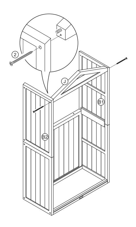
Assemble the upper back panel (I) to the shed assembly.
