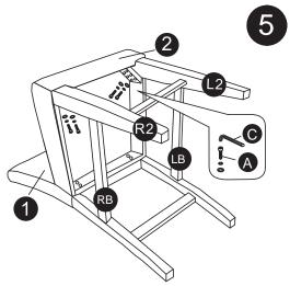
Put the screws in the holes, tight the screws, but not too tight, 90% is ok.
