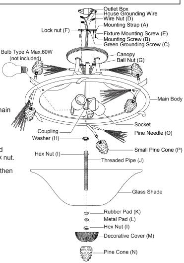
7. Attach the fixture to the mounting strap by inserting two fixture mounting screws, and then secure it with two ball nuts.
