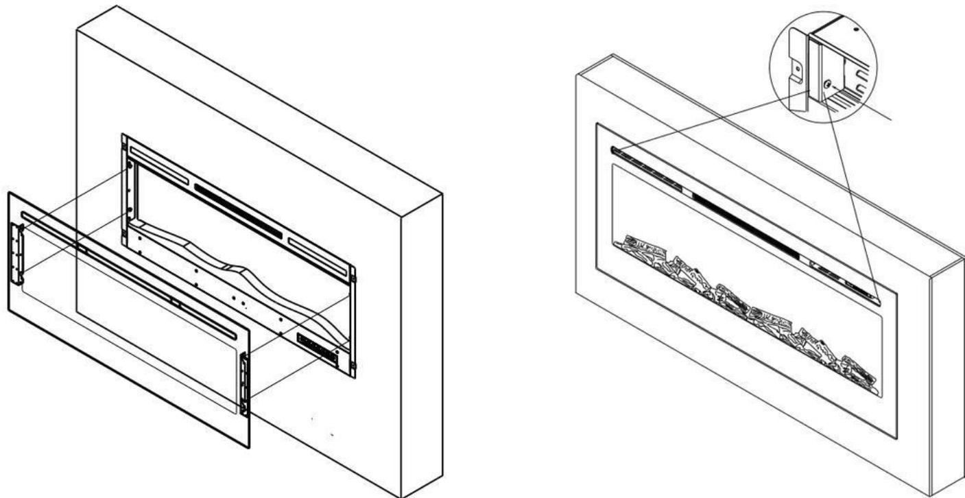
For the 86273/86277, reinstall screws 1 and 2.
