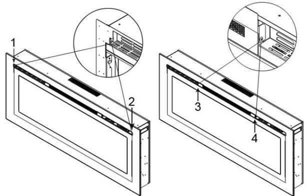
B – Remove screws in the vent opening
