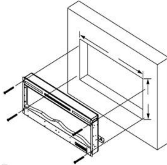
4. Once the fireplace is installed in the wall, place crystal embers or fire log in the fireplace.
