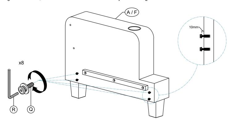
Step 7: Raise the Front/Back Panels (C) up , bring the Front/Back Panels (C) and align the hook on the side rail to the bolts. Once the Front/Back Panels (C) is set, tighten all bolts by using a Allen key (R). After assembly, re-tighten all bolts for a snug fit. DO NOT OVER TIGHTEN.
