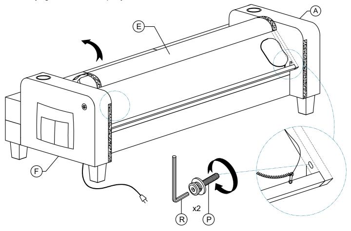
Step 13: After securing the 2 bolts at the bottom, rotate the Backest Frame (E) and install to Armrest (A / F) by Bolts 5/16" x 50mm (P) with Allen Key (R).
