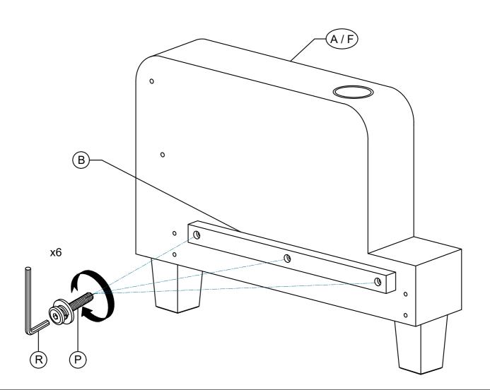
Step 6: Insert Bolts 1/4" x 25mm (Q) with Allen Key (R) on the Armrests by manually. NOTE: Do not fully tighten the bolts, leave at least 10mm visible so that you can hanger hook on the bolts.
