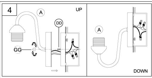
4. Attach fixture (A) to screws (DD) use ball nuts (GG) to Secure tightly.
