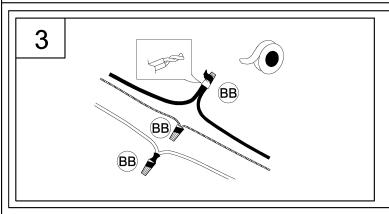
3. Strip 3/8" of insulation from the electrical wire ends. Using wire nuts (BB), connect white fixture wire to the white supply wire from the outlet box; connect the black fixture wire to the black supply wire.
