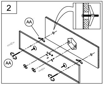
2. Attach assembled parts from step 1 on the wall, use the toggle bolt (AA) and the mounting screws supplied with the outlet box to secure tightly (not included).
