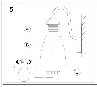
5. Attach glass shades (B) to fixture (A) use socket rings (C) to secure tightly.
