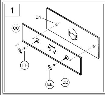
1. Place back plate (CC) on wall and use a pencil to mark the locations of the 2 mounting holes. Remove the back plate from the wall. Drill (2) Ø5/8" (Ø15.9mm) holes for mounting with toggle.
