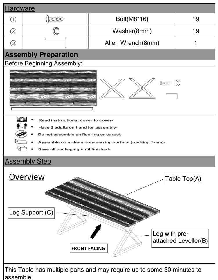
To give you an overview of the Table parts, the above picture is to help you put the various parts into perspective.
