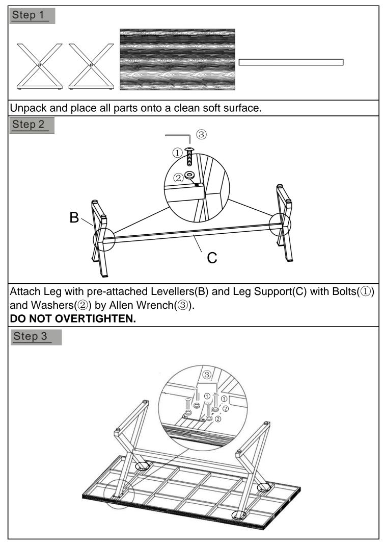
Turn the table top upside down to a soft surface to avoid scratching. Attach Table Leg with Pre-attached Levellers(B) to the mounting position on the table top(A) with Bolts(1), Washers(2) by Allen Wrench(3). **DO NOT OVERTIGHTEN.**
