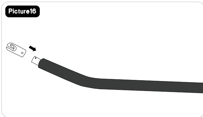
Install the all Tube Cap (#18) onto the all Steel Upper Net Pole with Foam (#8).
