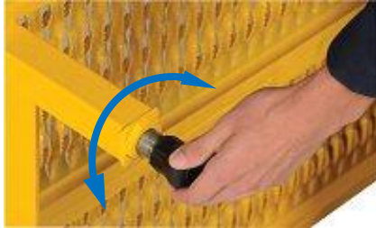
Turn leg counterclockwise to increase platform height
