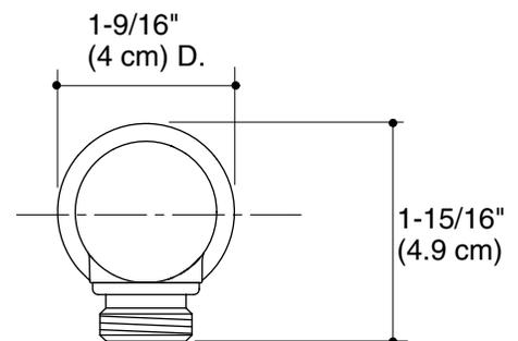
For NPT connection, nipple must extend 9/16" (1.4 cm) beyond finished wall.
