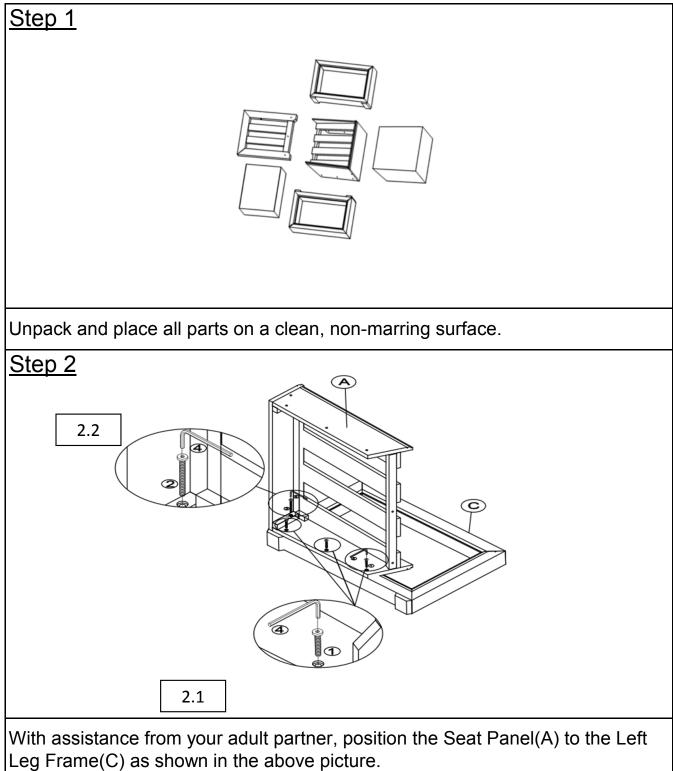
2.1) Using 3 Bolts((1)), with the Allen Key((4)), attach the Seat Panel(A) to the Left Leg Frame(C) as pictured.
