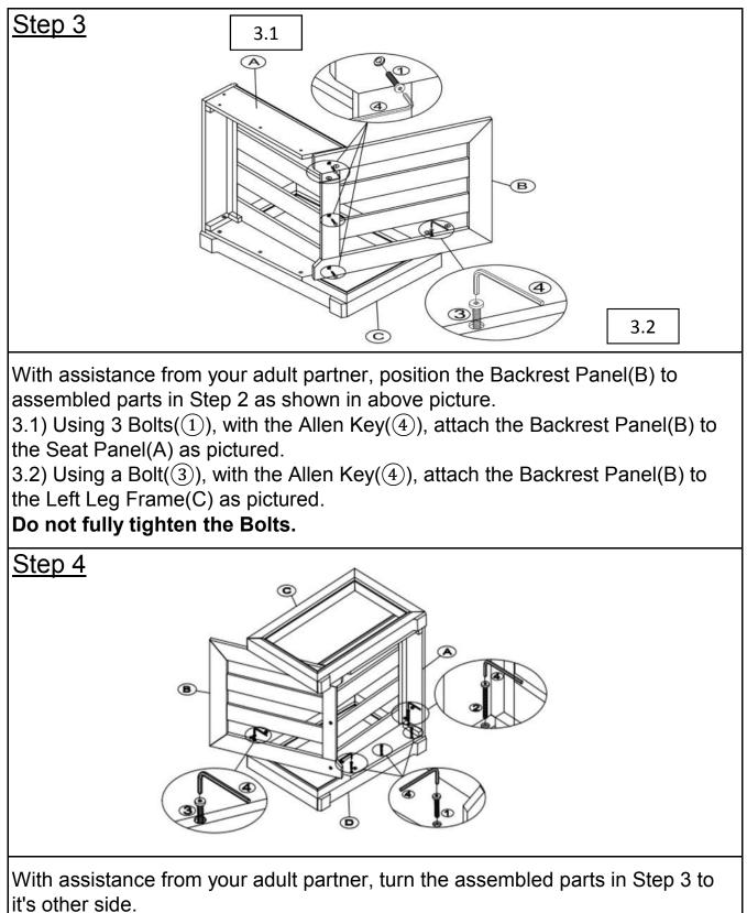
Repeat the same process in Step 2 and 3 to attach the Right Leg Frame(D) to the Seat Panel(A) and the Backrest Panel(B).
