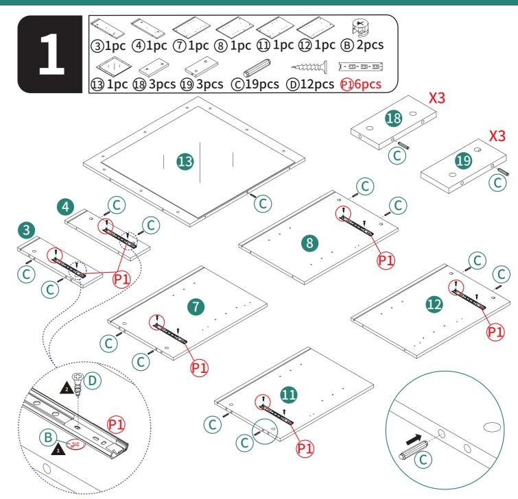
Note: Installing the slide will block the hole of part B (eccentric wheel), so it is recommended to first install part B (eccentric wheel) into its corresponding hole before installing the slide. This will facilitate step 9.
