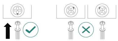
Quickfit head should be in the centre of the cam lock when the two panels are joined. Cam lock should be inserted before quickfit.
