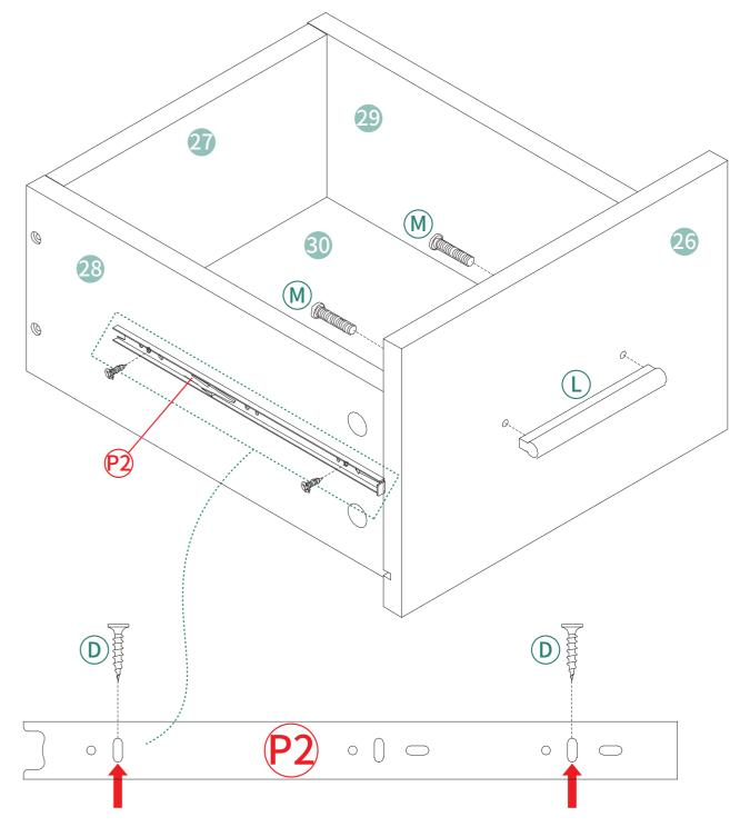
Align the screws with the center of the mounting hole of the guide rail.
