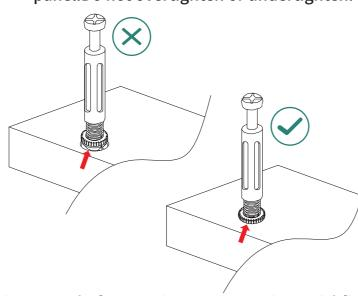
When fitting cam lock, ensure starting position is correct before you insert connecting quickfit.
