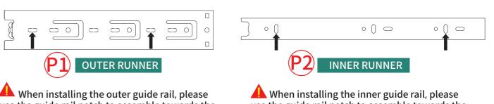
When installing the outer guide rail, please use the guide rail notch to assemble towards the inner direction of the drawer. Please fix the screws according to the marked position. If the installed position is changed, adjust it side-to-side at the marked position.
