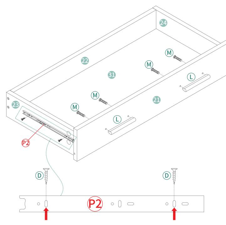
Align the screws with the center of the mounting hole of the guide rail.
