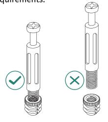
Tighten quickfit until shoulder is flush with panel.Do not overtighten or undertighten.
