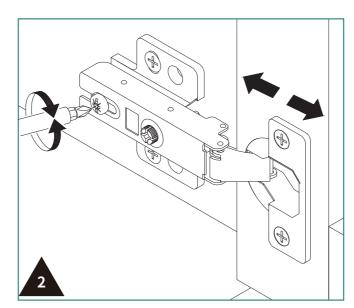
3. Use the screw at the front end of the hinge to adjust the left and right position of the door panel (ensure that the left and right sides of the door panel are in the same plane as the upper and lower panels).
