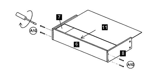
Attach the drawer head with secure by Mini Fix 12mm (F1). Assemble 4 sets of drawer in repeated at step 3.
