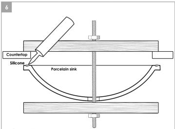
Clamp the boards so the sink stays suspended about 1 in below the countertop. Clean sink flange and underside of cut-out area of countertop, making sure that the area is smooth and free of debris. Apply continuous bead of silicone caulk evenly on top of sink flange.
