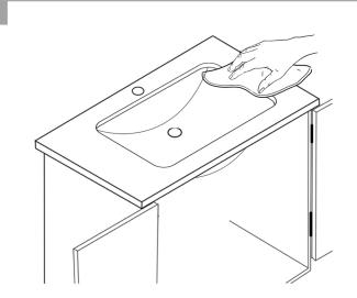
Wipe away excess silicone caulk with damp cloth. Connect drain and water supply according to manufacturer's instruction.
