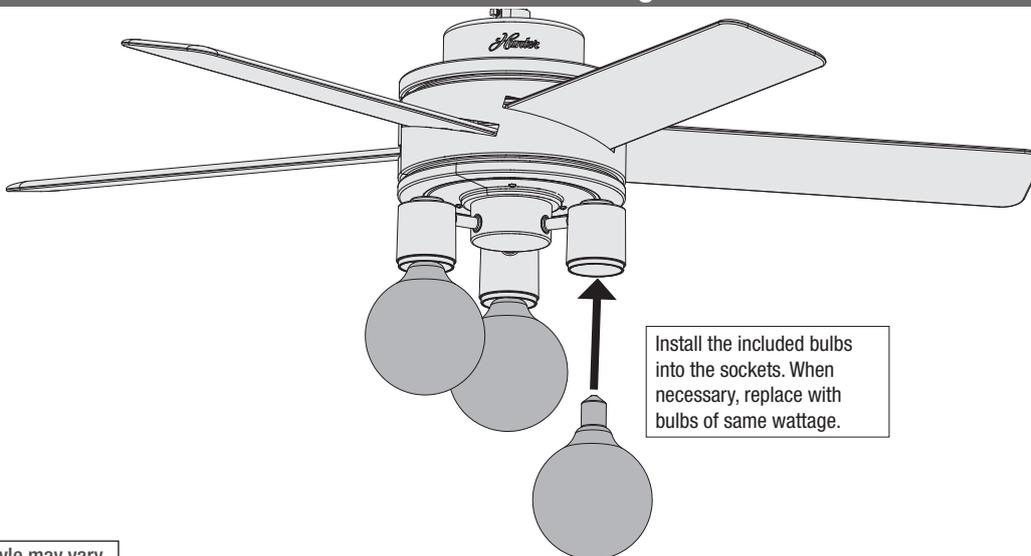
Install the included bulbs into the sockets. When necessary, replace with bulbs of same wattage.
