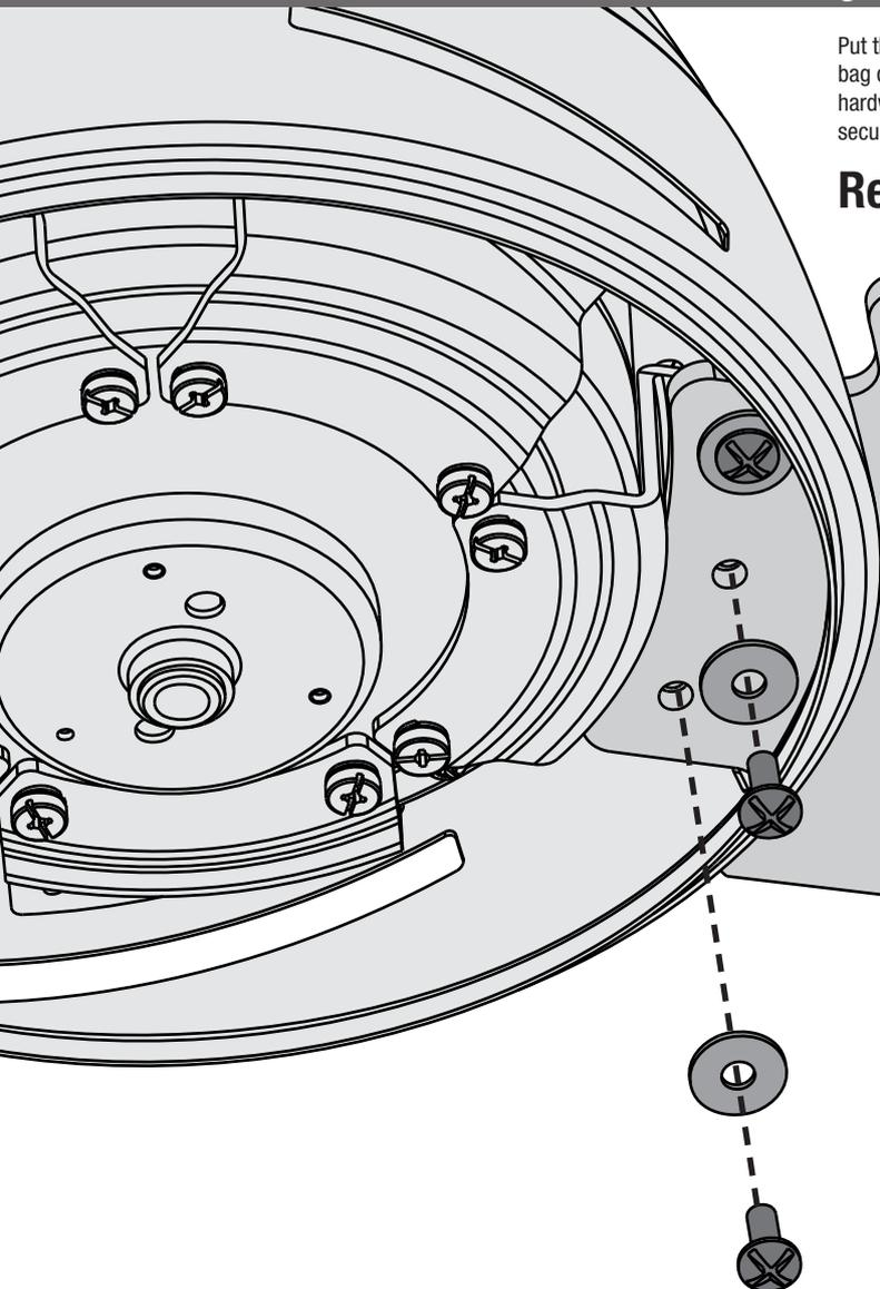
Put the blade washers found in the ■ hardware bag onto the blade screws found in the ▲ hardware bag. Then install the blade screws to secure each blade to the fan.
