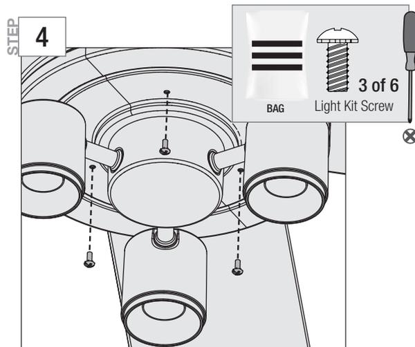
Install the three switch housing screws, found in the hardware bag. Tighten all three screws.
