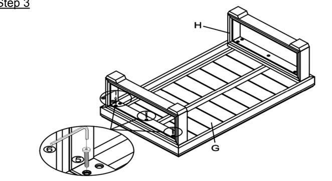
Attach the remaining Leg Frame(H) to the Table Top(G) using Bolts((5)) and the Allen Key(6).
