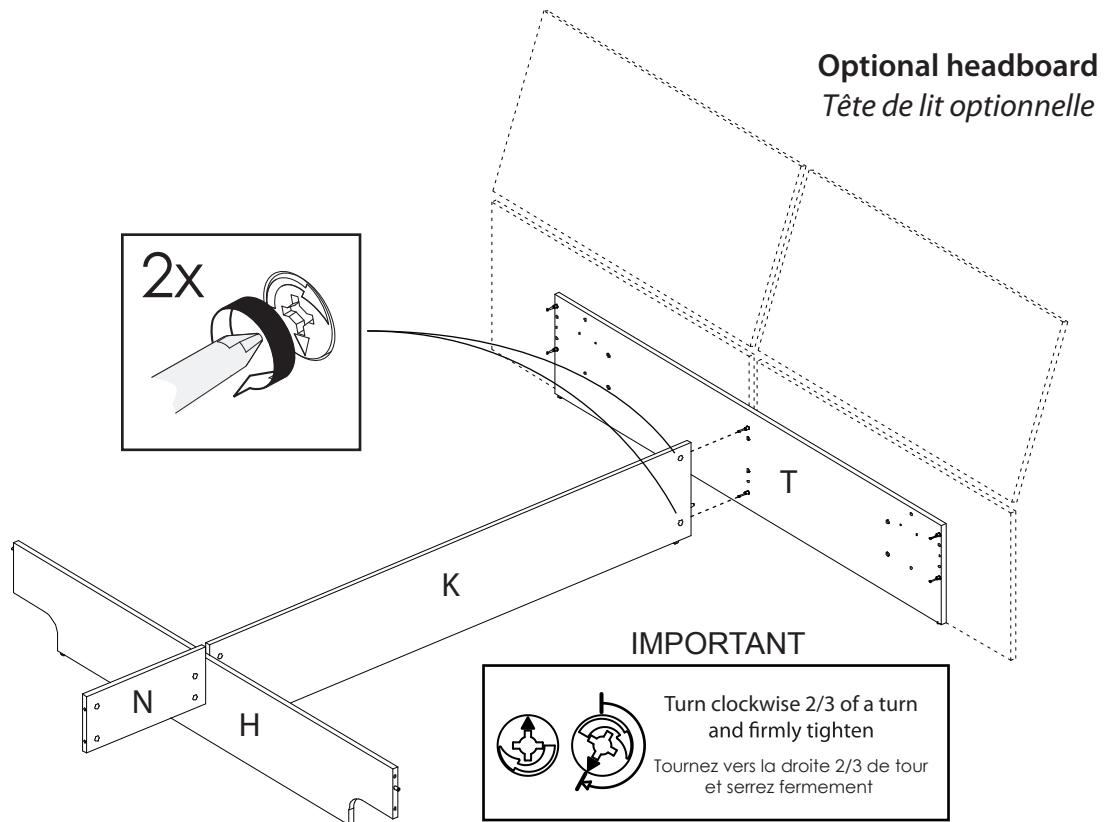
**8** Fasten the 2 panels B to the panels H and T. Then, tighten the 8 cam locks # 0203 located on the panel H and both panels B
