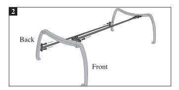
Step 2. Base assembly. Holding base frame sections in place, attach base crossmembers as shown in illustration 2 using two stainless steel short bolts for each side. Tighten.
