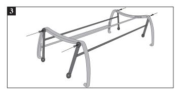
Step 3. Attach the swing bars to the outside of the base frame as shown using the stailess steel long bolts.
