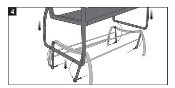
Step 4. Lower the completed seat section carefully over the base. Using the stainless steel long bolts, attach the seat side frame to the lower ends of the swing bars. Note that the section of the base frame containing the lowest crossmember bar is the back side.
