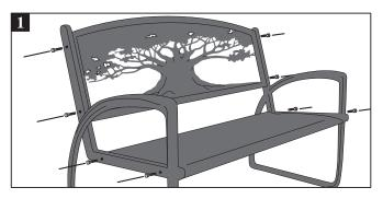
Step 1. Seat assembly. Holding the side frame sections in place, attach the backrest with the black bolt/washer/nut combos. Do not tighten. Position the seat section in place and secure with the remaining black hardware, then tighten all bolts.
