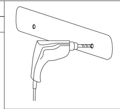
2. Mark the location of the mounting holes on the wall, also mark or measure the location of the pedestal, it is recommended that for additional safety, a piece of 1" x 4" x 23" piece of lumber be preinstalled underneath the console to provide additional support.
