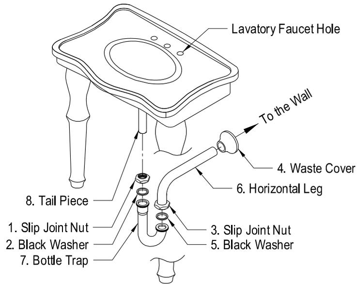
1. Remove horizontal leg and slip joint nut from bottle trap.
