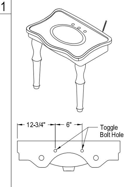
1. Gently place basin on top of pedestal legs and very carefully place in the location where the console will be installed.
