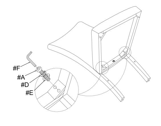
Do not tighten screws until completely asembled.
