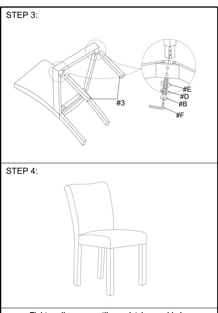
Tighten all screws until completely asembled.
