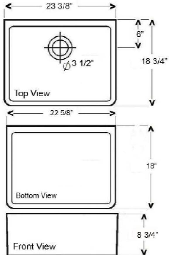
Dimensions of fixture are nominal and may vary within the range of tolerances established by ANSI Standard A112.19.2.2013. Dimensions and specifications subject to change without notice.
